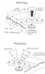
Figure 14-11. Schematic diagram illustrating the writing and reading processes in a programmable multilayer magneto-optic disk. (From Ref. 25 with permission from Elsevier Sequoia S.A.).
